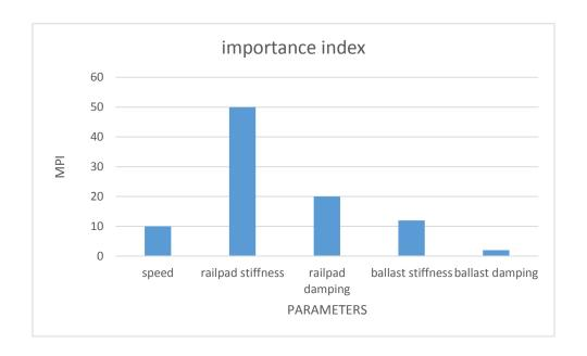
After performing the differential analysis, an uncertainty analysis is made by applying the Monte Carlo methodology. This takes into account a great number of evaluations using different configurations over the parameter space. Once the simulations are done the mean and standard deviation of the evaluations is used to obtain the uncertainty in the model predictions and the input variables that generate the mentioned uncertainty.
