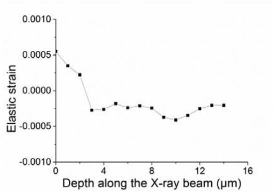
Fig 2: The residual strain along longitudinal direction at a depth of 6.5mm.
