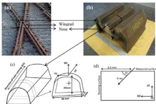
Fig 1 : Illustration showing where the measurements were done.
