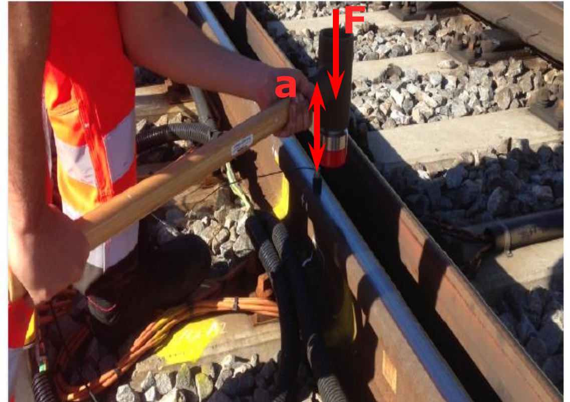
Setup for the receptance test including hammer and accelerometers
